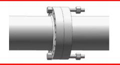
**3.** Insert the wedge into the joint until the heel of the step is in contact with the outer surface of the joint.
