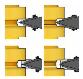
To remove the Stepped Blocks unscrew the M6 countersunk screw. Do not force the screw out of the Stepped Block, it is deliberately retained to prevent it becoming misplaced.
