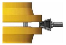
The wedges can then be retracted fully and inserted again, using the next step. In this way the flange joint can be iteratively opened further until the required spread is reached.
