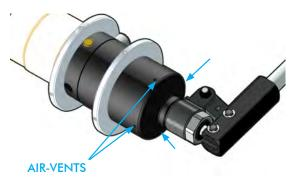
The TFA integral hydraulic tools use a hydraulic cylinder to advance the Alignment Piston and align the flanges. The hydraulic pressure is applied using the integrated hand pump, enabling accurate control of the force applied.
