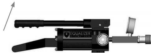
3. The pump handle is depressed, which pumps the oil from the chamber through the outlet port and into the system to which the pump is connected
