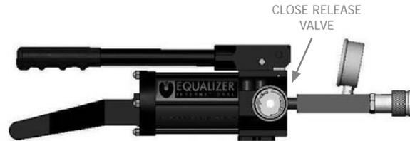
2. The pump handle is raised, which creates a vacuum in the piston chamber which sucks oil from the reservoir into the chamber
