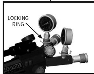
2. Ensure the hydraulic systems you wish to pressurise have been bled and are free from air and leaks. Connect the pump into the systems using the screw connectors supplied with the pump, push the male and female connectors together fully and rotate the locking rings clockwise until fully tight.
