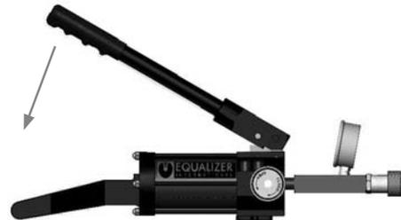
4. Steps 2 & 3 are repeated, which will pump oil into the system until the maximum pressure of 10,000 psi (700 bar) is achieved, at which point the safety release valve will open and the oil will cycle back to the reservoir
